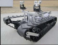
All of The Machine Lab's basic platforms come with motors, proportional motor controllers, batteries, quadrature encoders, external charge jack and LED fuel gage. The MMP-40X also has accessable on board power distribution with 5V and 12V, 3 amp regulated outputs to power other devices such as radio receivers, micro controllers, video equipment servos or sensors or other equipment.
