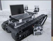
A modular 80/20 rail system can easily be implimented to mount equipment, sensors, laptops or mechanical accessories. (sold separately)
